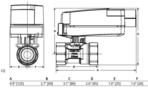
Modulating, Electrical fail-safe, 24 V
